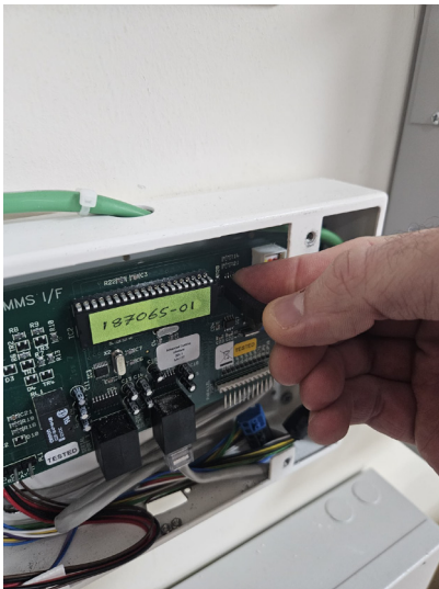
4. Rotate the remover tool round to be vertical so it prises against the PCB
